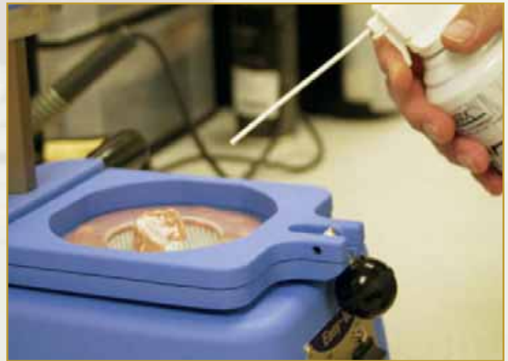
Figure 7: Freeze Spray with the Vacuum Machine
