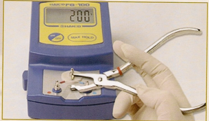
Figure 16: Testing Temperature with Thermometer
