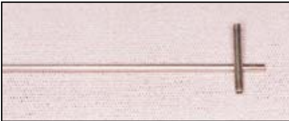
Fig. 1 Two sections of .040" stainless steel tubing spot-welded together prior to soldering.
